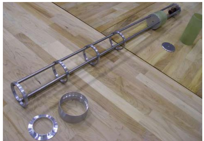
The most essential element of the first Drake design, as fabricated by Eric Haberman. Three steel rods form the motor/sabot rack. The actuating piston and Rouse CD3 unit are on the upper right.
