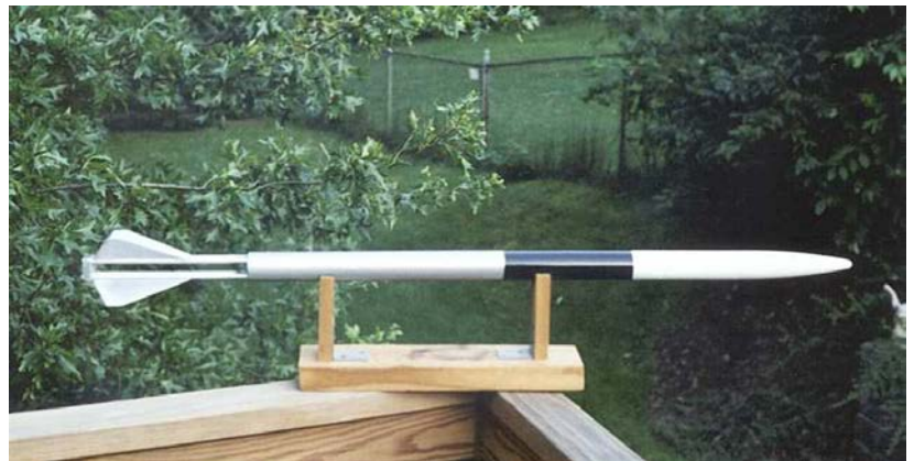
Above: The Bellerophon – a three or four-stage aluminum dowel rod rack-rocket designed to fly on single-use 24 mm D/E/F motors.
