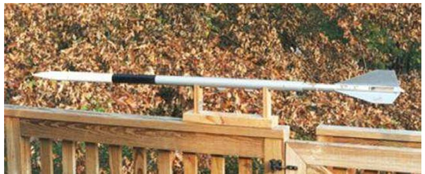
Below: The Exeter II – a three stage rack-rocket designed to fly on single-use 29 mm F/G motors. In this case, the dowel rod “rack” is replaced by an aluminum tube, with 5/8” wide slots cut into the tube to open the motor stack area and defeat the “Krushnik Effect.”
