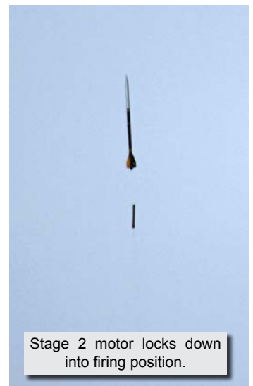
Stage 1 motor clears the end of the airframe.
