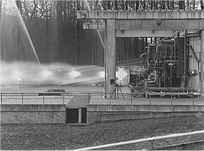
FIGURE 20–4. Visible plume created by the oxygen–hydrogen propellants of the Vulcain 60 thrust chamber, with a specific impulse of 439 sec at altitude, a nozzle expansion area ratio of 45, and a mixture ratio of 5.6. The upstream portions of the diamonds of the multiple shock wave patterns are visible in the core of the plume because of emissions from reacting minor species. (Courtesy of EADS Astrium, Germany.)
