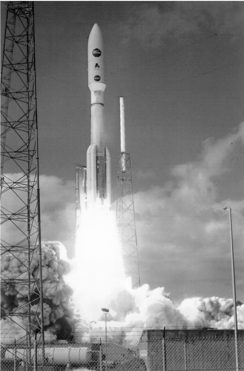
FIGURE 1–13. Atlas V space launch vehicle with three (or five) strap-on stages using Aerojet solid rocket motors and a central Energomash (Russia) RD-180 liquid propellant booster rocket engine running on LOX/kerosene. (Courtesy Lockheed Martin Corp.)
