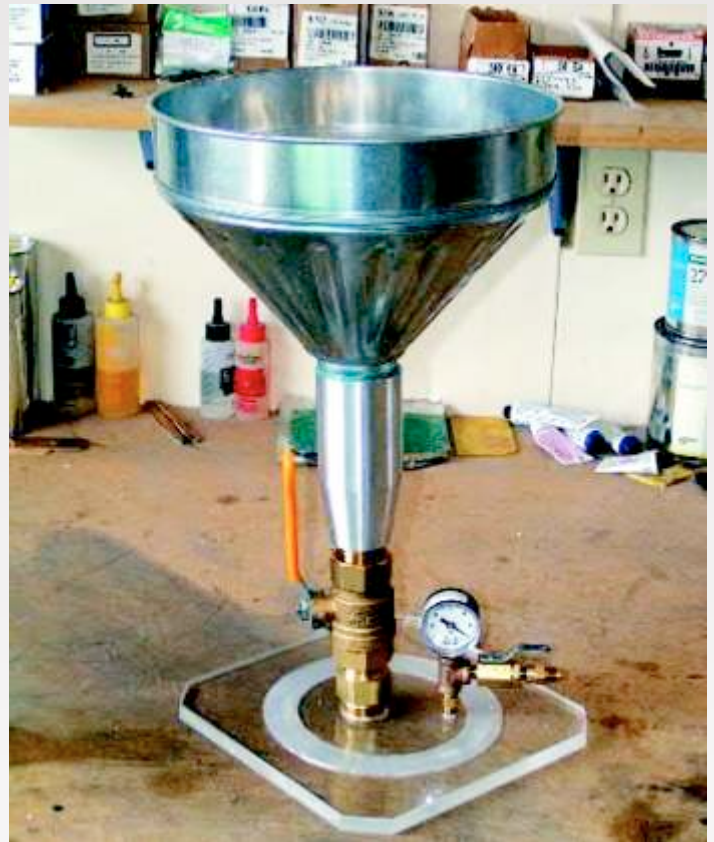
The heart of the whole operation is the top plate. Just about self explanatory it resembles a large standard Vacuum Plate with a big funnel attached.
