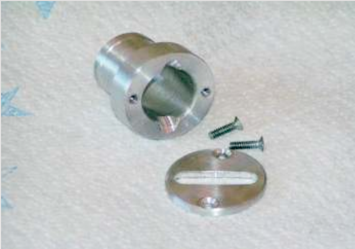
The Do-Dad is designed in two pieces for cleaning purposes and possible future modifications.
