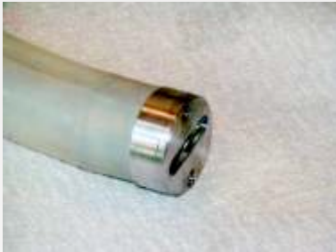
The "Do-Dad" piece is attached to the end of the flexible tubing. A hose clamp (not shown) assures it staying on during vacuum.
