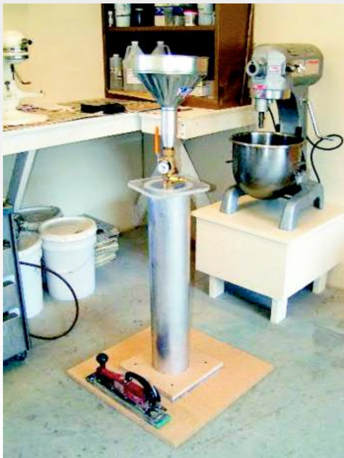
A complete working Vacuum Casting Machine capable of filling a 6" diameter Casting Tube is simple and workable.
